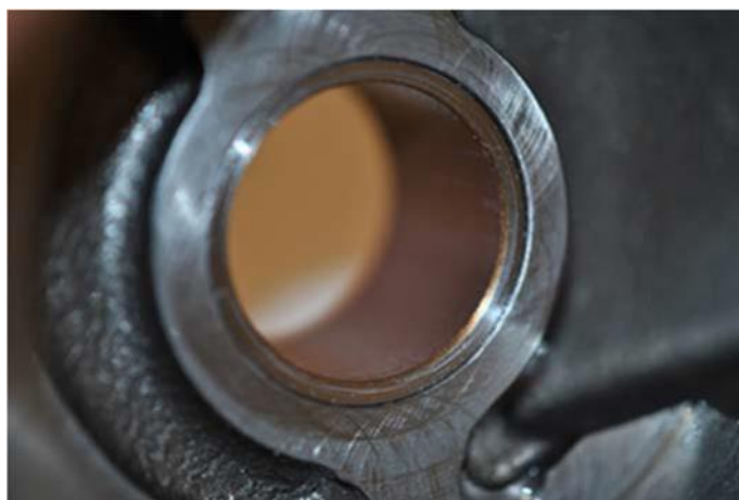
Figure 2 Photograph of DP31 bearing following Cascon's HALT Testing (Highly Accelerated Life Test).
