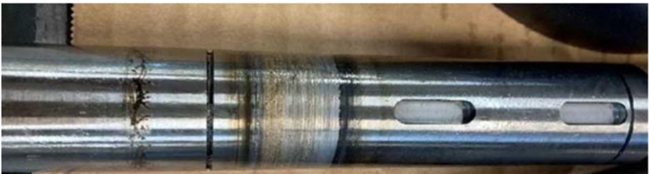
Figure 1 Representative damaged pump hardware. Top: Inner and outer gerotor and housing showing wear on face of inner gerotor. Middle: Wear on DU bearing. Bottom: Wear of shaft adjacent to DU bearing.
